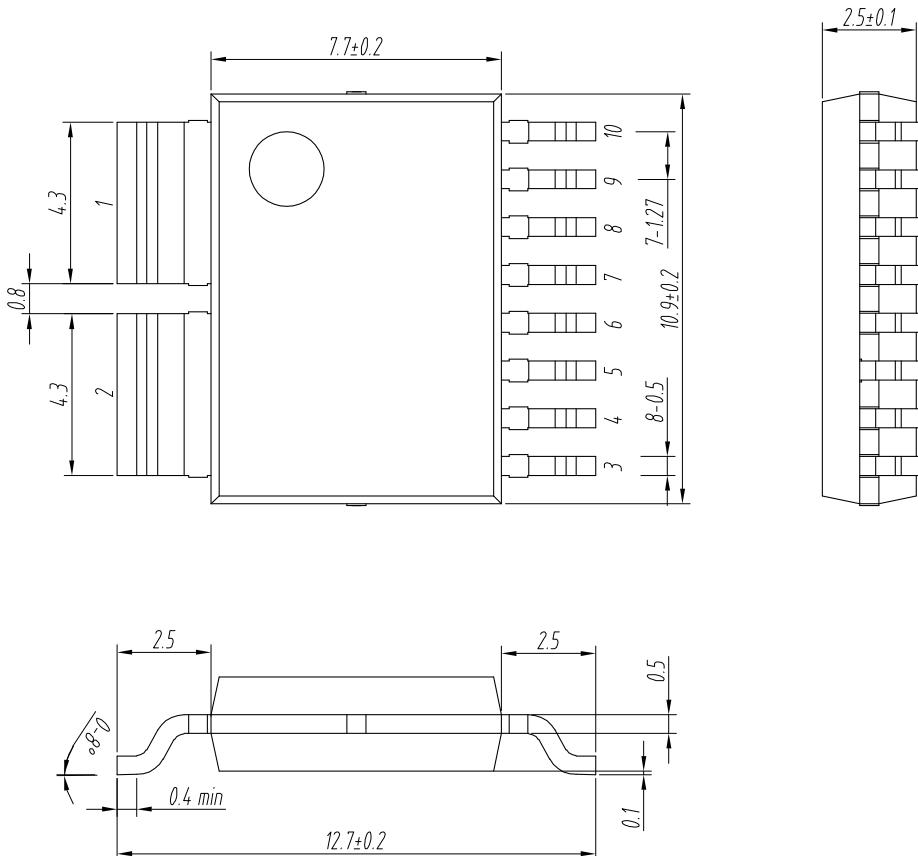
Figure 2. Dimensions of STK-616AM3 series sensors. The unit is mm.
