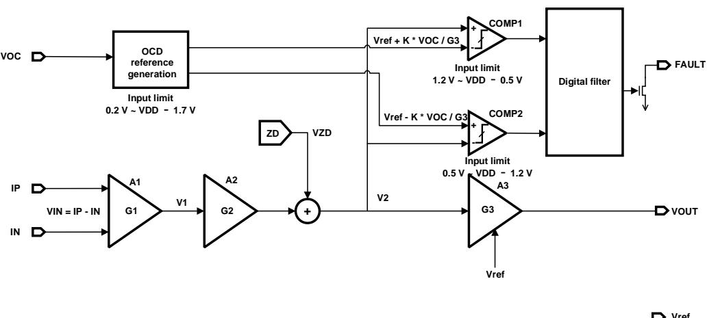
Figure 11 the functional block diagram for STK-616AM3 on OCD function with conditions of  $V_{cc} = 5$  V,  $V_{off} = 2.5$  V,  $V_{ref} = 2.5$  V.
