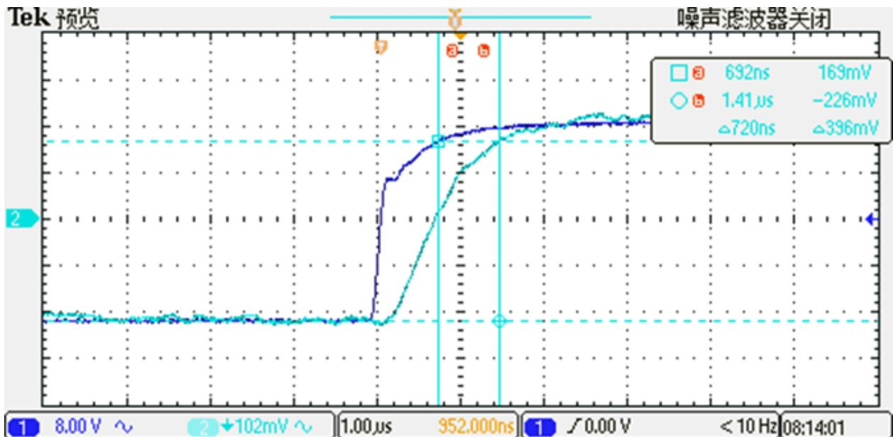
Figure 5. The typical frequency response of STK-616AM3 series current sensor. The response time from 90% of the primary current to 90% of the secondary output is 0.9μs.
